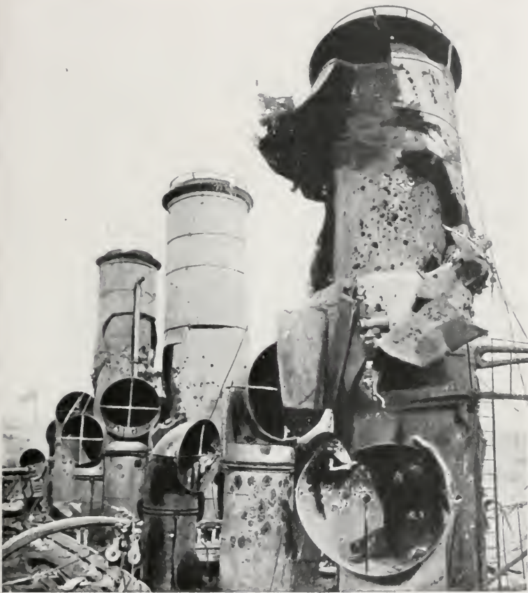
THE FUNNELS OF THE "VINDICTIVE", ON HER RETURN FROM ZEEBRUGGE. After being summarily repaired, the "Vindictive" accomplished her last exploit, by blowing up Ostend Harbour on May 11, 1918. (See page 68).
